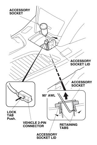
7. Push the lock tab in and disconnect the vehicle 2-pin connector from the accessory socket.
