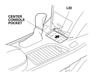
Open the accessory socket lid. Remove the accessory socket by reaching in the driver's console trim opening and pushing up on the accessory socket. Use a 90° awl to release the two retaining tabs.
